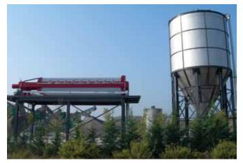
Filterpress and deep cone thickener tank
